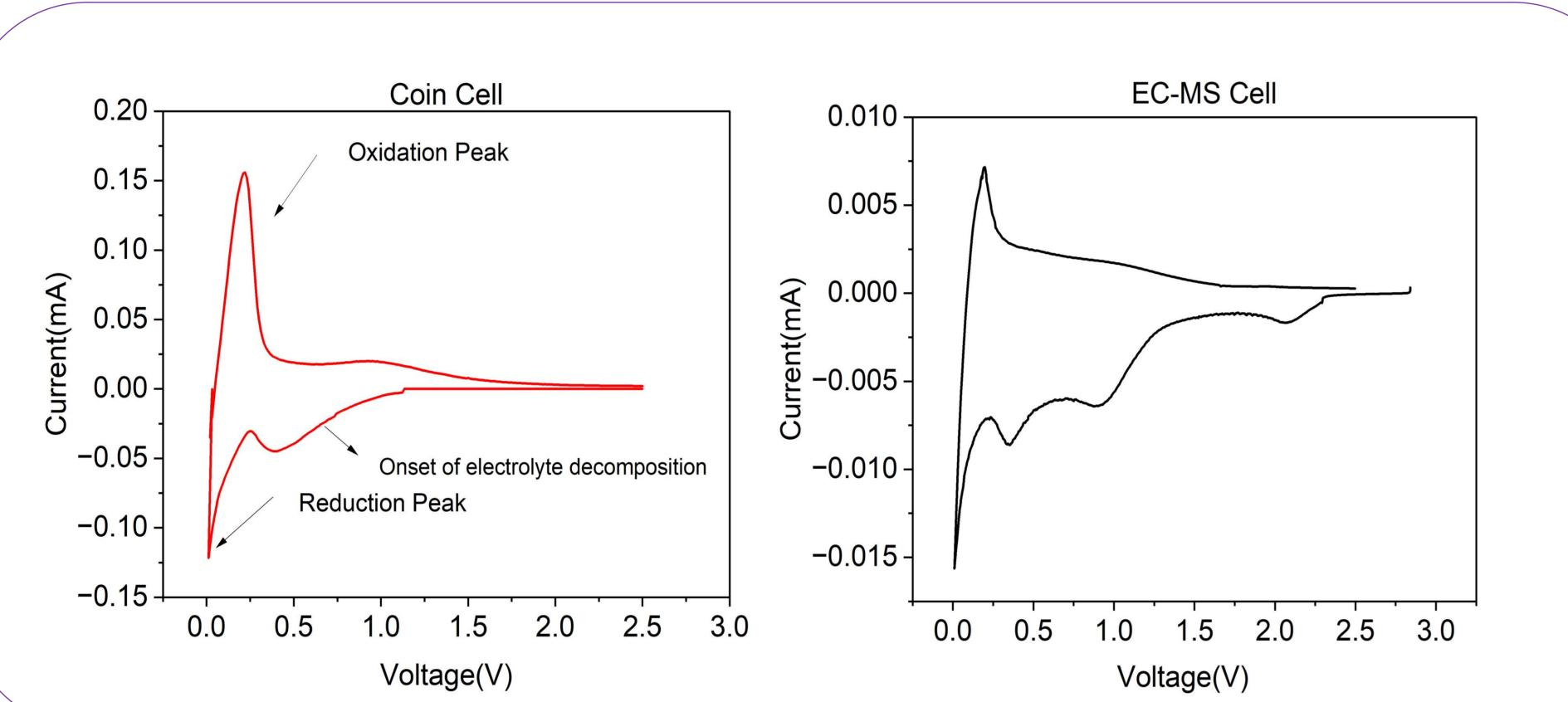
**Electrolyte-** NaPF<sub>6</sub> EC:DEC Working Electrode- Hard Carbon **Counter Electrode-** Na Metal
