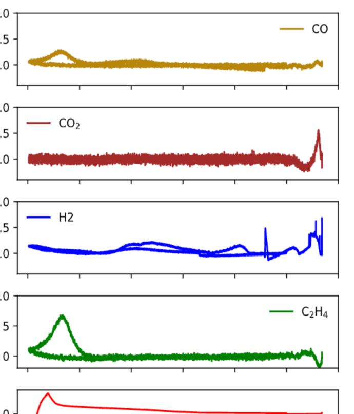
CO Corresponding to decomposition of ethylene carbonate to form the SEI.  $C_3H_4O_3 + 2Na^+ + 2e^- \longrightarrow COM_a + CO$
